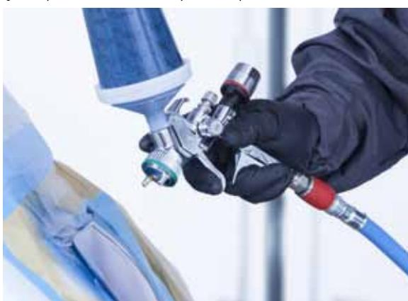
The SATAmijet 4400 B is perfectly suitable for application on smaller surfaces – in both craft and industry
