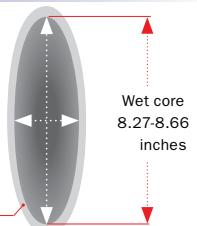
Standard nozzles with wet, compact core. SR nozzles with wide-stretched core.
