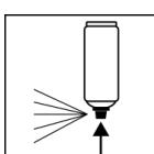
After painting, turn the can upside down and spray the valve until empty.
