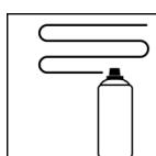
Dry film thickness 20 - 30 µm
