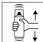
After filling, shake can thoroughly for at least 2 minutes from when the mixing balls are heard.
