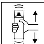
Shake can thoroughly for at least 2 minutes from when the mixing balls are heard.
