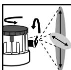
Set the variable spray nozzle to the size and pattern of the damage.
