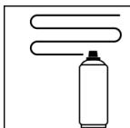
Dry film thickness 15 - 30 µm
