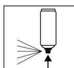
After painting, turn the can upside down and spray the valve until empty.
