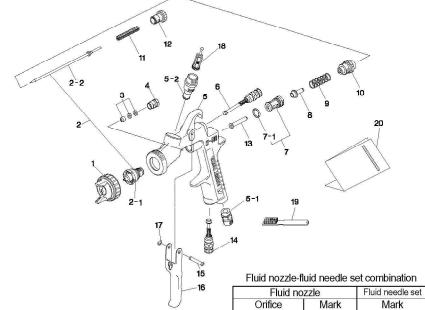
Orifice  $\phi$  mm(in) W200/12 40012 φ1.2(0.047) W200/13  $\phi$  1.3(0.051) 20015 φ1.4(0.055) W400/14 W400/16 φ1.6(0.063) W20018 φ 1.8(0.071) W200/18 φ2.5(0.098) W200/25 W20025
